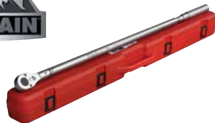
MTN16600 3/4 in. Drive 100-600 Ft/lbs. Torque Wrench • Click style torque wrench with PRO ratchet head • Micrometer style clicks and/or releases when preset torque is reached • Hardened steel body with knurled handles • Complies with ASME and federal specifications • 1 year warranty on material and workmanship
