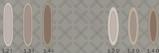
Fan pattern shape I and O nozzle HVLP/RP
