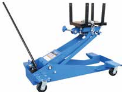
KTI63517A $1,769.99 1.5 Ton Truck Trans Jack (HD) • Low height: 7-4/5" • High height: 36-1/2" • Chassis Length: 43-1/2"; Chassis Width: 26 • Saddle Tilt 10 degrees • 2 year warranty on material & workmanship
